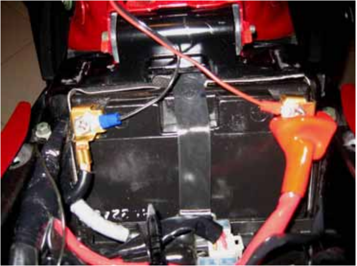
Power supply cable wires connected to motorcycle's battery
